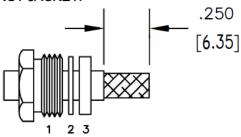
2. FORM BRAID OVER CLAMP NUT (4). TRIM BRAID BACK TO SHOULDER. CUT DIELECTRIC & CENTER CONDUCTOR TO DIMENSION SHOWN. DO NOT NICK CENTER CONDUCTOR. SOLDER CONTACT TO CENTER CONDUCTOR. REMOVE EXCESS SOLDER. DO NOT OVER HEAT DIELECTRIC. INSERT CABLE ASSEMBLY INTO BODY & TIGHTEN.
