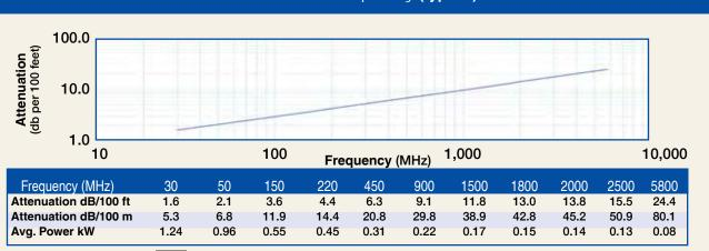
Calculate Attenuation = (0.290501) • √FMHz + (0.000396) • FMHz (interactive calculator available at http://www.timesmicrowave.com/cable\_calculators)
