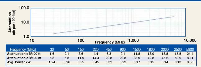
Calculate Attenuation =  $(0.290501) \bullet \sqrt{FMHz} + (0.000396) \bullet FMHz$  (interactive calculator available at http://www.timesmicrowave.com/cable\_calculators)
