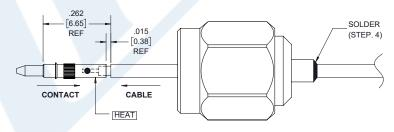
USING ASSEMBLY TOOL, PRESS CONTACT FULLY INTO INSULATOR. SOLDER OUTER CONDUCTOR TO BODY.
