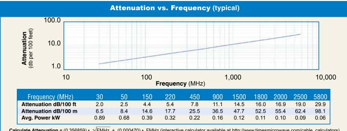
Calculate Attenuation = (0.356859) • √FMHz + (0.000470) • FMHz (interactive calculator available at http://www.timesmicrowave.com/cable\_calculators)
