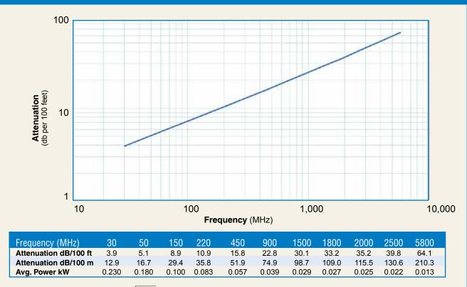
Calculate Attenuation = (0.709140) •  $\sqrt{FMHz}$  + (0.001740) • FMHz (interactive calculator available at http://www.timesmicrowave/telecom) Attenuation: VSWR=1.0 ; Ambient = +25°C (77°F) Power: VSWR=1.0; Ambient = +40°C; Inner Conductor = 100°C (212°F); Sea Level; dry air; atmospheric pressure; no solar loading
