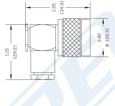
2. FORM BRAID OVER CLAMP NUT (4). CUT DIELECTRIC TO DIMENSION SHOWN. DO NOT NICK CENTER CONDUCTOR. SLIDE ASSEMBLY INTO BODY, SOLDER CENTER CONDUCTOR IN PLACE & TIGHTEN CLAMP NUT. SCREW CAP DOWN INTO PLACE.
