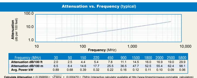
Calculate Attenuation = (0.356859) • √FMHz + (0.000470) • FMHz (interactive calculator available at http://www.timesmicrowave.com/cable\_calculators) Attenuation: VSWR=1.0; Ambient = +25°C (77°F) Power: VSWR=1.0; Ambient = +40°C; Inner Conductor = 100°C (212°F); Sea Level; dry air; atmospheric pressure; no solar loading
