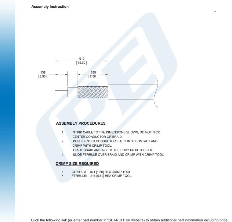
inventory and certifications: BNC Male Connector Crimp/Crimp Attachment for RG58, RG303, RG141, PE-C195, PE-P195, LMR-195, 0.195 inch PE4016
