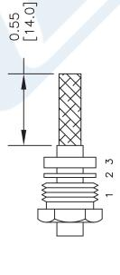
FORM BRAID OVER CLAMP NUT (4). TRIM BRAID CONTACT TO CENTER CONDUCTOR, REMOVE CENTER CONDUCTOR TO DIMENSION SHOWN. DO NOT NICK CENTER CONDUCTOR, SOLDER DIELECTRIC, INSERT CABLE ASSEMBLY INTO BACK TO SHOULDER, CUT DIELECTRIC & **EXCESS SOLDER, DO NOT OVER HEAT** BODY & TIGHTEN, 7
