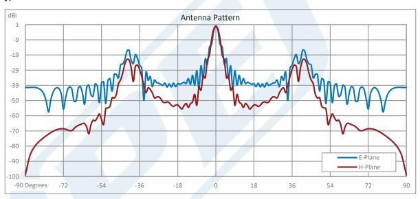
Click the following link (or enter part number in "SEARCH" on website) to obtain additional part information including price, inventory and certifications: WR-12 Waveguide Lens Horn Antenna Operating from 72 GHz to 82 GHz with a Nominal 37 dBi Gain with UG-387/U Round Cover Flange PEWAN1080
