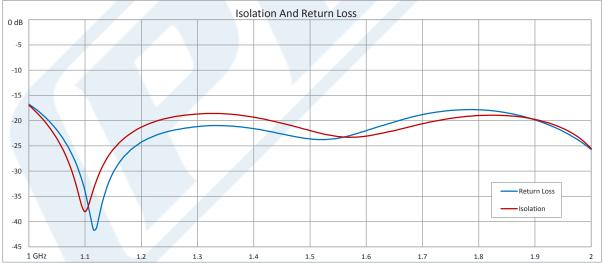
Click the following link (or enter part number in "SEARCH" on website) to obtain additional part information including price, inventory and certifications: High Power Circulator with 18 dB Isolation from 1 GHz to 2 GHz, 100 Watts and SMA Female PE83CR1000
