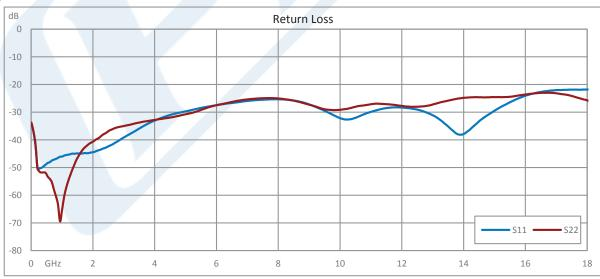
Click the following link (or enter part number in "SEARCH" on website) to obtain additional part information including price, inventory and certifications: DC Block on Outer Conductor SMA Male to SMA Female Operating From 10 MHz to 18 GHz PE8211
