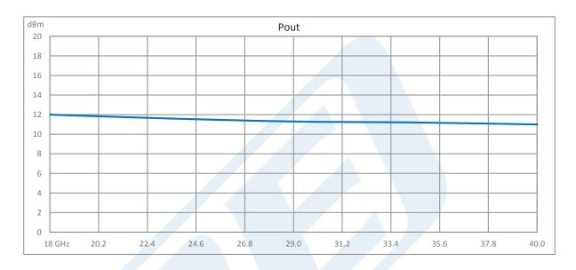
High Power Limiter, Field Replaceable 2.92mm, 100W Peak Power, 15 us Recovery, 13 dBm Flat Leakage, 18 GHz to 40 GHz from Pasternack Enterprises has same day shipment for domestic and International orders. Our RF, microwave and millimeter wave products maintain a 99.4% availability and are part of the broadest selection in the industry.
