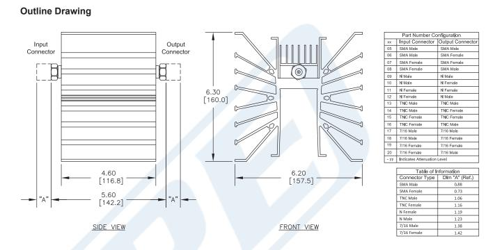
6 dB Fixed Attenuator, SMA Female To SMA Male Directional Black Aluminum Heatsink Body Rated To 300 Watts Up To 3 GHz from Pasternack Enterprises has same day shipment for domestic and International orders. Our RF, microwave and millimeter wave products maintain a 99% availability and are part of the broadest selection in the industry.
