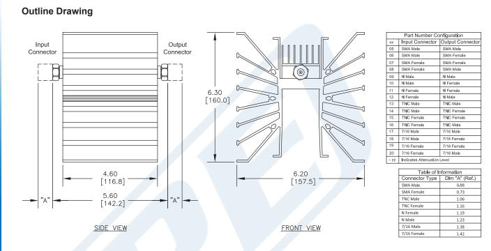
30 dB Fixed Attenuator, SMA Female To SMA Male Directional Black Aluminum Heatsink Body Rated To 300 Watts Up To 3 GHz from Pasternack Enterprises has same day shipment for domestic and International orders. Our RF, microwave and millimeter wave products maintain a 99% availability and are part of the broadest selection in the industry.
