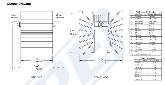
3 dB Fixed Attenuator, SMA Female To SMA Male Directional Black Aluminum Heatsink Body Rated To 300 Watts Up To 3 GHz from Pasternack Enterprises has same day shipment for domestic and International orders. Our RF, microwave and millimeter wave products maintain a 99% availability and are part of the broadest selection in the industry.
