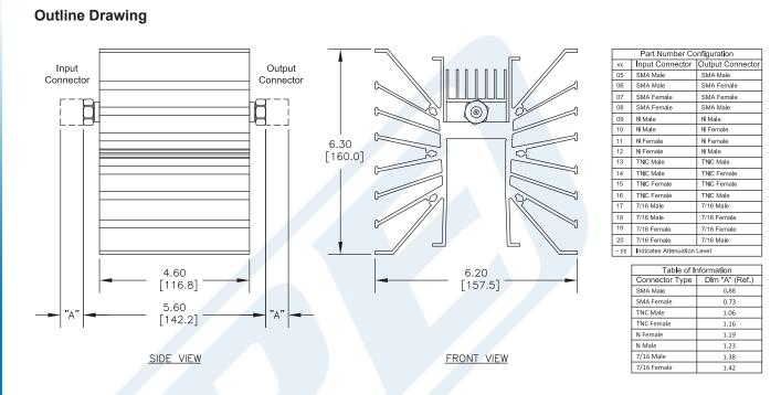
6 dB Fixed Attenuator, SMA Female To SMA Female Directional Black Aluminum Heatsink Body Rated To 300 Watts Up To 3 GHz from Pasternack Enterprises has same day shipment for domestic and International orders. Our RF, microwave and millimeter wave products maintain a 99% availability and are part of the broadest selection in the industry.
