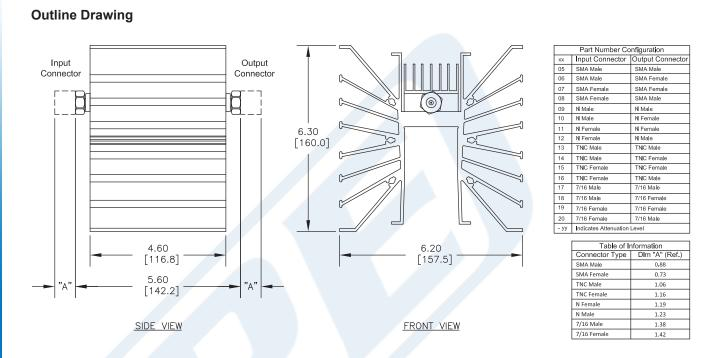
50 dB Fixed Attenuator, SMA Female To SMA Female Directional Black Aluminum Heatsink Body Rated To 300 Watts Up To 3 GHz from Pasternack Enterprises has same day shipment for domestic and International orders. Our RF, microwave and millimeter wave products maintain a 99% availability and are part of the broadest selection in the industry.
