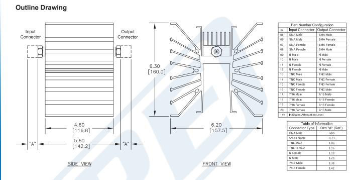
30 dB Fixed Attenuator, SMA Female To SMA Female Directional Black Aluminum Heatsink Body Rated To 300 Watts Up To 3 GHz from Pasternack Enterprises has same day shipment for domestic and International orders. Our RF, microwave and millimeter wave products maintain a 99% availability and are part of the broadest selection in the industry.
