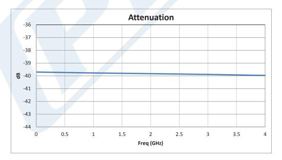
Click the following link (or enter part number in "SEARCH" on website) to obtain additional part information including price, inventory and certifications: 40 dB Fixed Attenuator, SMA Male to SMA Female Black Anodized Aluminum Heatsink Body Rated to 25 Watts Up to 4 GHz PE7393-40
