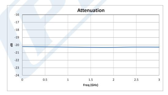
Click the following link (or enter part number in "SEARCH" on website) to obtain additional part information including price, inventory and certifications: 20 dB Fixed Attenuator, SMA Male to SMA Female Aluminum Body Rated to 5 Watts Up to 3 GHz PE7391-20
