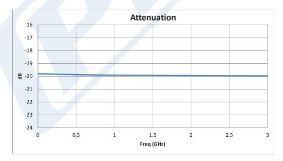
Click the following link (or enter part number in "SEARCH" on website) to obtain additional part information including price, inventory and certifications: 20 dB Fixed Attenuator, N Male to N Female Black Anodized Aluminum Heatsink Body Rated to 50 Watts Up to 3 GHz PE7389-20
