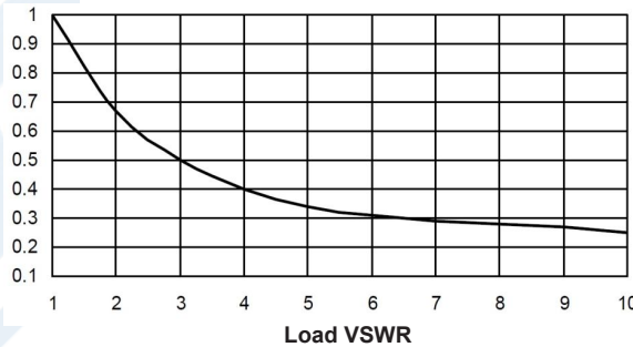
Power Handling De-rating vs. Load VSWR
