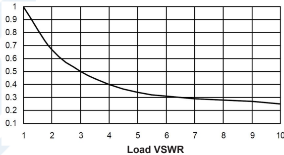
Power Handling De-rating vs. Load VSWR
