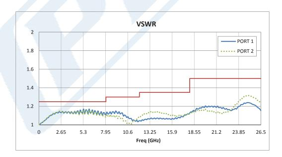
Click the following link (or enter part number in "SEARCH" on website) to obtain additional part information including price, inventory and certifications: SPDT Electromechanical Relay Failsafe Switch DC to 26.5 GHz, SMA, 20 Watts, 28V Control PE71S6095
