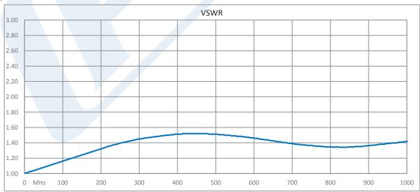
Click the following link (or enter part number in "SEARCH" on website) to obtain additional part information including price, inventory and certifications: 75 Ohm A/B Coaxial Electromechanical Relay Switch, DC to 1,000 MHz, 5W, 12V, BNC PE7101
