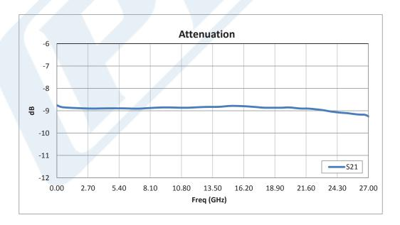
Click the following link (or enter part number in "SEARCH" on website) to obtain additional part information including price, inventory and certifications: 9 dB Fixed Attenuator, SMA Male to SMA Female Passivated Stainless Steel Body Rated to 2 Watts Up to 26 GHz PE7087-9
