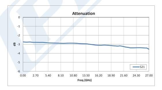
Click the following link (or enter part number in "SEARCH" on website) to obtain additional part information including price, inventory and certifications: 3 dB Fixed Attenuator, SMA Male to SMA Female Passivated Stainless Steel Body Rated to 2 Watts Up to 26 GHz PE7087-3
