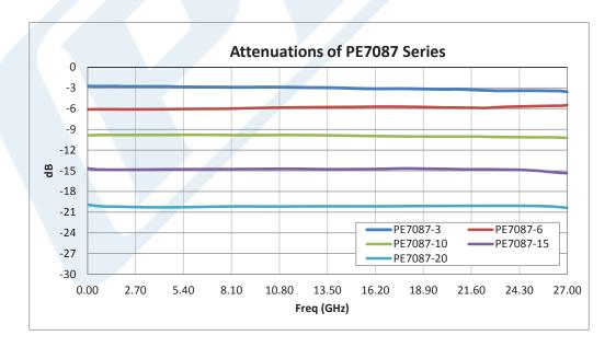
Click the following link (or enter part number in "SEARCH" on website) to obtain additional part information including price, inventory and certifications: 0 dB Fixed Attenuator, SMA Male to SMA Female Passivated Stainless Steel Body Rated to 2 Watts Up to 26 GHz PE7087-0
