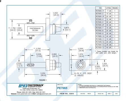
0 to 10 dB Rotary Continuously Variable Attenuator, SMA Female To SMA Female Rated To 5 Watts From 12.4 GHz To 18 GHz from Pasternack Enterprises has same day shipment for domestic and International orders. Our RF, microwave and millimeter wave products maintain a 99% availability and are part of the broadest selection in the industry.
