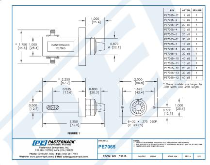
0 to 40 dB Rotary Continuously Variable Attenuator, SMA Female To SMA Female Rated To 5 Watts From 8 GHz To 12.4 GHz from Pasternack Enterprises has same day shipment for domestic and International orders. Our RF, microwave and millimeter wave products maintain a 99% availability and are part of the broadest selection in the industry.
