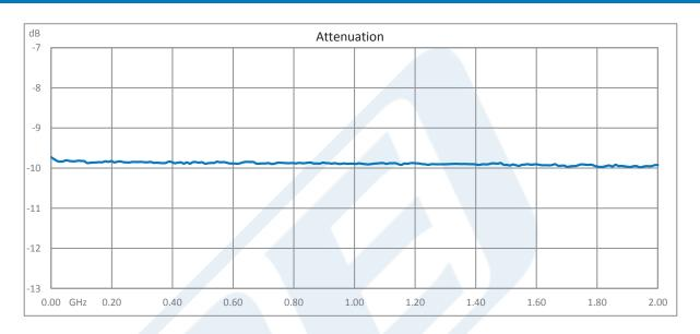
10 dB Fixed Attenuator, TNC Male to TNC Female Brass Nickel Body Rated to 1 Watt Up to 2 GHz from Pasternack Enterprises has same day shipment for domestic and International orders. Our RF, microwave and millimeter wave products maintain a 99.4% availability and are part of the broadest selection in the industry.
