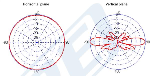
Fixed Antenna Operates From 2.4 GHz to 2.5 GHz With a Typical 8 dBi Gain N Female Input Connector IP67 Rated from Pasternack Enterprises has same day shipment for domestic and International orders. Our RF, microwave and millimeter wave products maintain a 99.4% availability and are part of the broadest selection in the industry.
