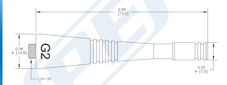
Click the following link (or enter part number in "SEARCH" on website) to obtain additional part information including price, inventory and certifications: Whip Antenna Operates From 880 MHz to 960 MHz With a Typical 0 dBi Gain SMA Female Input Connector IP67 Rated PE51165
