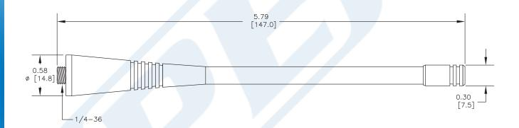
Click the following link (or enter part number in "SEARCH" on website) to obtain additional part information including price, inventory and certifications: Whip Antenna Operates From 698 MHz to 870 MHz With a Typical 2 dBi Gain SMA Female Input Connector IP67 Rated PE51154
