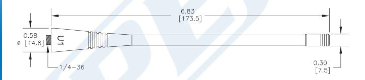
Click the following link (or enter part number in "SEARCH" on website) to obtain additional part information including price, inventory and certifications: Whip Antenna Operates From 400 MHz to 420 MHz With a Typical 0 dBi Gain SMA Female Input Connector IP67 Rated PE51145
