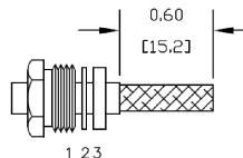
2. FORM BRAID OVER CLAMP NUT (4). TRIM BRAID BACK TO SHOULDER. CUT DIELECTRIC & CENTER CONDUCTOR TO DIMENSION SHOWN. DO NOT NICK CENTER CONDUCTOR. SOLDER CONTACT TO CENTER CONDUCTOR. REMOVE EXCESS SOLDER. DO NOT OVER HEAT DIELECTRIC. INSERT CABLE ASSEMBLY INTO BODY & TIGHTEN WITH TORQUE 26-30 in-lbs.
