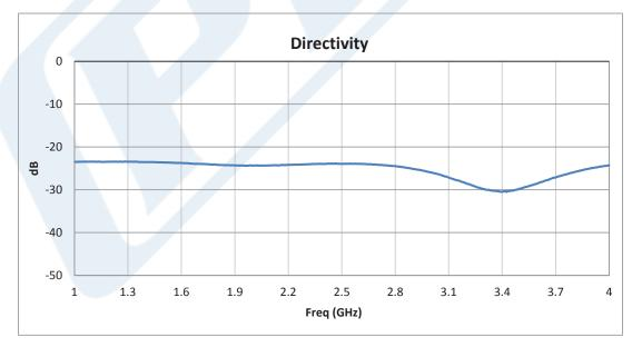
Click the following link (or enter part number in "SEARCH" on website) to obtain additional part information including price, inventory and certifications: Directional 6 dB SMA Coupler From 1 GHz to 4 GHz Rated to 50 Watts PE2209-6
