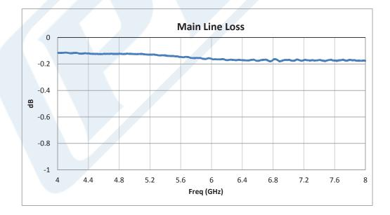
Click the following link (or enter part number in "SEARCH" on website) to obtain additional part information including price, inventory and certifications: Directional 30 dB SMA Coupler From 4 GHz to 8 GHz Rated to 50 Watts PE2204-30
