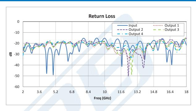
4 Way SMA Wilkinson Power Divider From 2 GHz to 18 GHz Rated at 10 Watts from Pasternack Enterprises has same day shipment for domestic and International orders. Our RF, microwave and millimeter wave products maintain a 99.4% availability and are part of the broadest selection in the industry.
