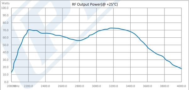
Click the following link (or enter part number in "SEARCH" on website) to obtain additional part information including price, inventory and certifications: 43 dB Gain, 20 Watt Psat, 2 GHz to 4 GHz, High Power GaN Amplifier, Class AB, SMA PE15A5119
