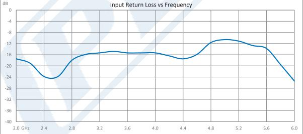
Click the following link (or enter part number in "SEARCH" on website) to obtain additional part information including price, inventory and certifications: 46 dB Gain, 40 Watt Psat, 2 GHz to 6 GHz, High Power GaN Amplifier, SMA, Class AB PE15A5067
