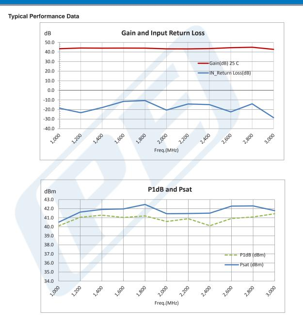
Click the following link (or enter part number in "SEARCH" on website) to obtain additional part information including price, inventory and certifications: 44 dB Gain, 8 Watt Psat, 1 GHz to 3 GHz, High Power GaAs Amplifier, SMA Input, SMA Output, 48 dBm IP3, Class AB, with Heatsink PE15A5037F
