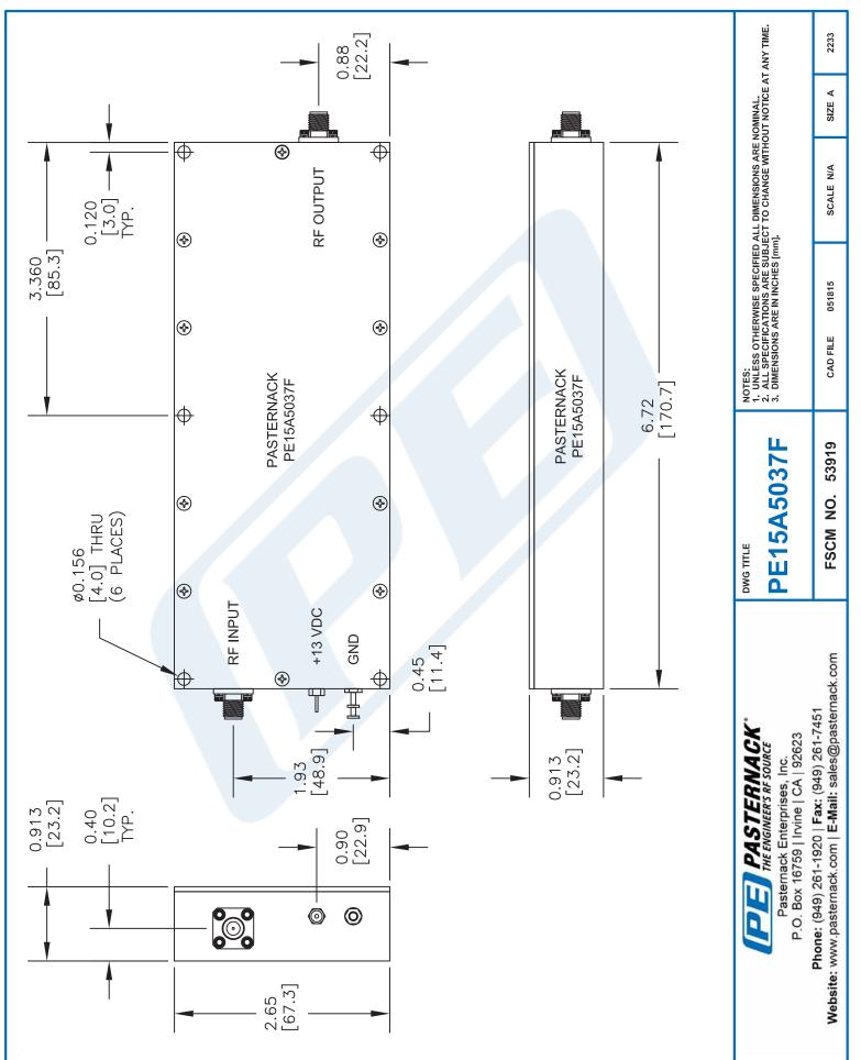
PE15A5037F CAD Drawing 44 dB Gain, 8 Watt Psat, 1 GHz to 3 GHz, High Power GaAs Amplifier,
