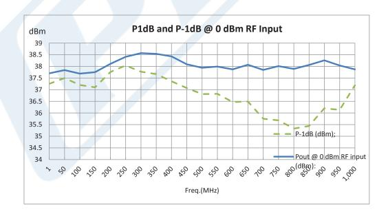
Click the following link (or enter part number in "SEARCH" on website) to obtain additional part information including price, inventory and certifications: 4 Watt Psat, 1 MHz to 1 GHz, High Power LDMOS Amplifier, SMA Input, SMA Output, 36 dB Gain, 39 dBm IP3, Class AB PE15A5030
