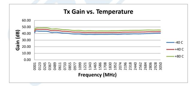
Click the following link (or enter part number in "SEARCH" on website) to obtain additional part information including price, inventory and certifications: 43 dB Gain, 10 Watt Psat, 30 MHz to 2.5 GHz, High Power GaN Amplifier, SMA PE15A5011
