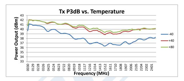
43 dB Gain, 10 Watt Psat, 30 MHz to 2.5 GHz, High Power GaN Amplifier, SMA from Pasternack Enterprises has same day shipment for domestic and International orders. Our RF, microwave and millimeter wave products maintain a 99.4% availability and are part of the broadest selection in the industry.
