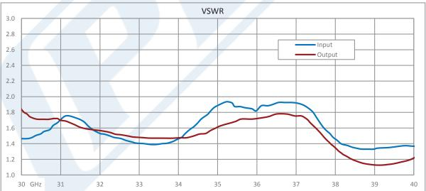
Click the following link (or enter part number in "SEARCH" on website) to obtain additional part information including price, inventory and certifications: 20 dBm Psat, 30 GHz to 40 GHz, Medium Power Amplifier with Heatsink, 2.92mm, 20 dB Gain PE15A4069F
