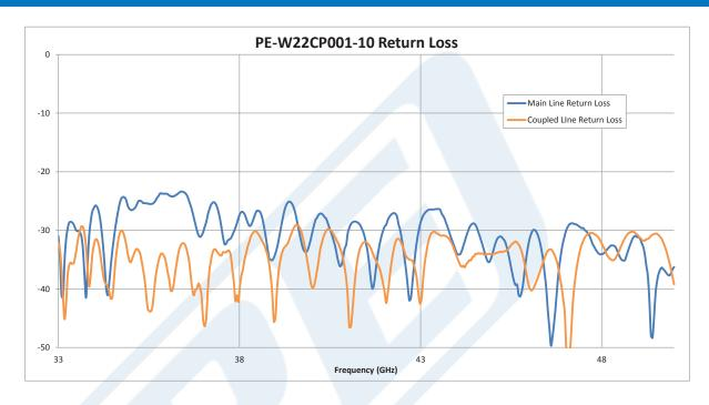
WR-22 Waveguide 10 dB Broadwall Coupler, UG-383/U Round Cover Flange, H-Plane Coupled Port, 33 GHz to 50 GHz, Brass Copper from Pasternack Enterprises has same day shipment for domestic and International orders. Our RF, microwave and millimeter wave products maintain a 99.4% availability and are part of the broadest selection in the industry.
