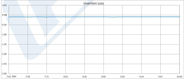
Click the following link (or enter part number in "SEARCH" on website) to obtain additional part information including price, inventory and certifications: WR-112 Seamless Flexible Waveguide 12 Inch, UG-51/U Square Cover Flange Operating from 7.05 GHz to 10 GHz PE-W112SF005-12
