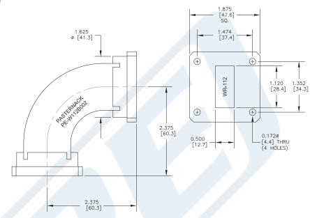
WR-112 Waveguide H-Bend with UG-51/U Flange Operating from 7.05 GHz to 10 GHz from Pasternack Enterprises has same day shipment for domestic and International orders. Our RF, microwave and millimeter wave products maintain a 99% availability and are part of the broadest selection in the industry.
